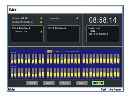
For normal operation green ticks should be present. A red cross means a problem has been detected and should be checked.
